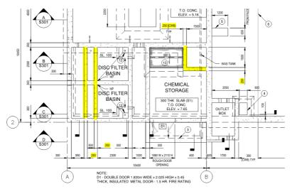
The walls in the Disc Filter Basin and Chemical Storage to all be CW7 (300mm). The scale will be corrected in the IFC set.
