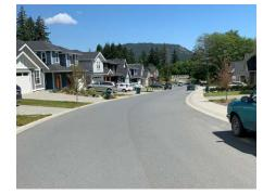
**Sidewalk, Unbuffered**Sidewalk facility that is directly adjacent the roadway.
