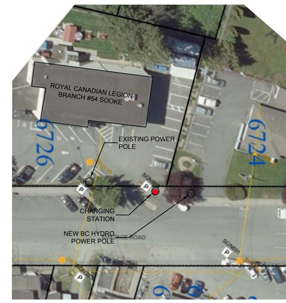
1 ELECTRICAL KEY PLAN E-001 SCALE: 1:500
