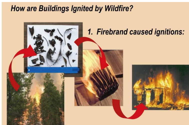
Figure 9. Firebrand caused ignitions: burning embers are carried ahead of the fire front and alight on vulnerable building surfaces.
