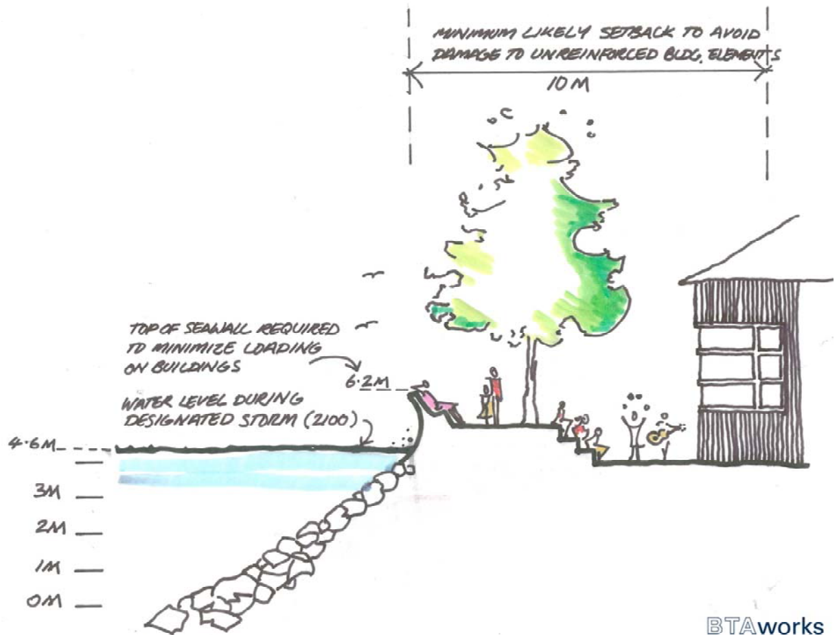
Figure 1-17: Example Sea Dike for 2100 – Granville Island source: BTAworks 1 elevations: CGD
